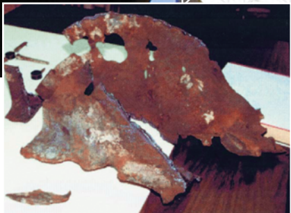
PREVIOUSLY MELTED STEEL FROM WTC 7 (THE SAME PIECE AS SHOWN ABOVE). THIS PHOTO IS TAKEN FROM APPENDIX C OF THE FEMA BUILDING PERFORMANCE STUDY.
