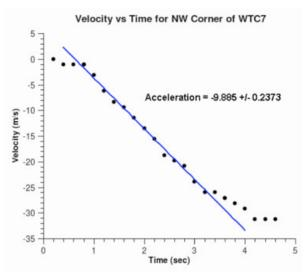
Figure 2: Velocity vs. Time for NW Corner of WTC 7
