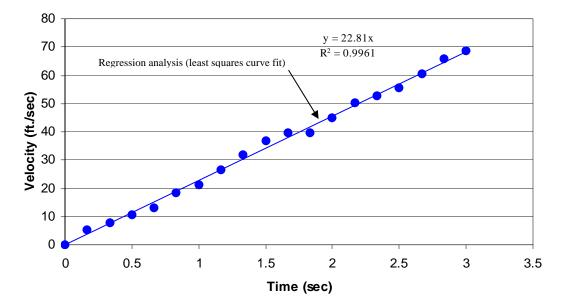
The velocity of the roof increases in a relatively linear way and is 68.65 ft./s after 3.00 seconds, which is about 71% of the free fall velocity of 96.52 ft./s for this fall time. At the actual measured distances and calculated velocities, the initial fall through one story would have taken place in approximately 1.0 second.
